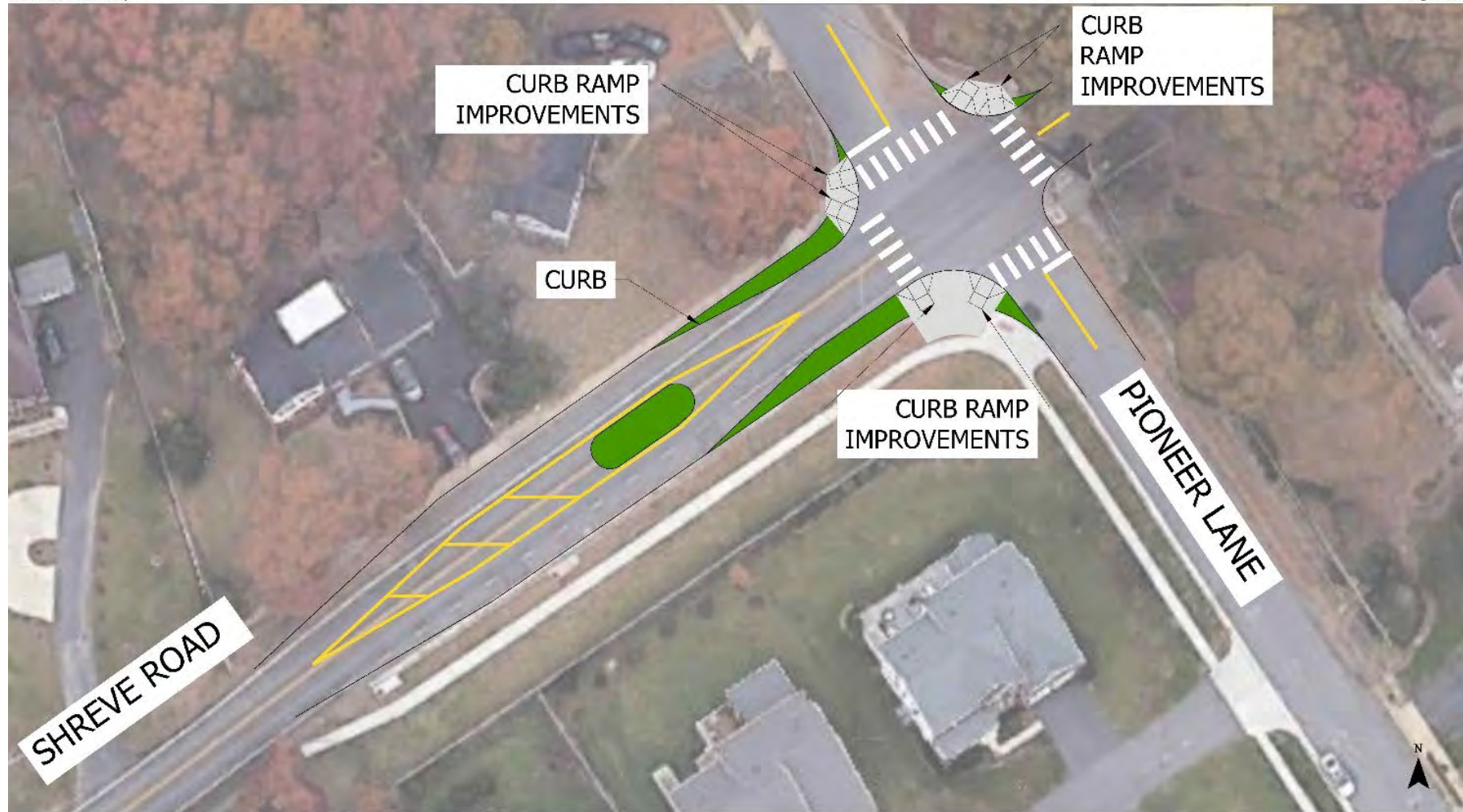
Idea 1 (Revised) - Chicane (Curb) Shreve Road at Pioneer Lane Shreve Road, VA
